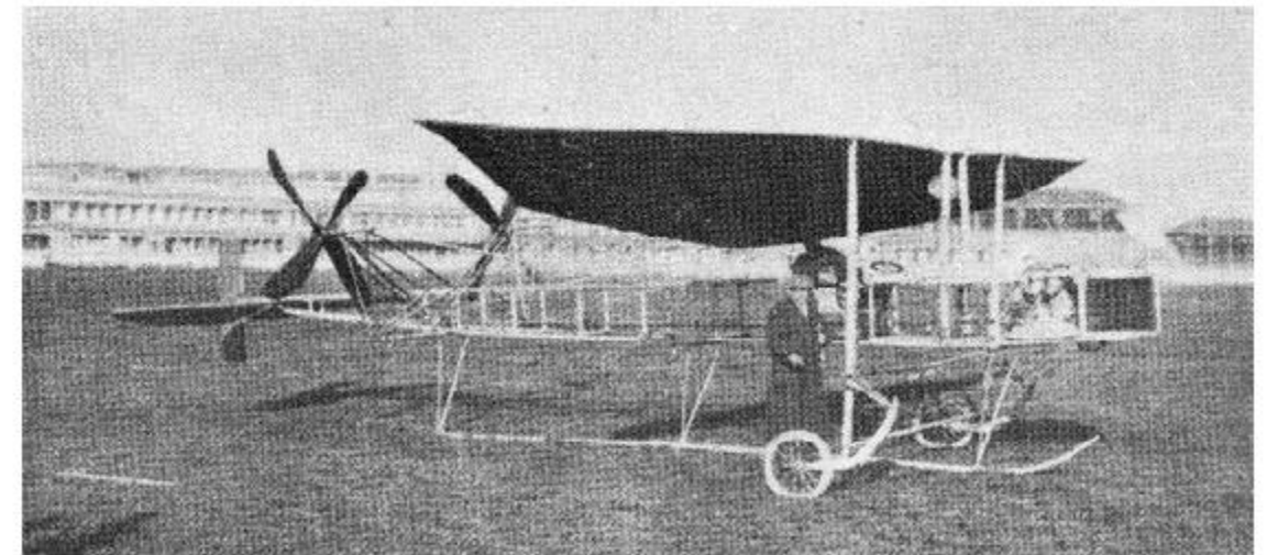
CHAUVIÈRE (1909-10). Attempt to develop a monoplane with propellers in rear. The idea has been resuscitated for some 1913 military monoplanes.
